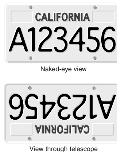
Figure 6. The view through a reflector telescope is rotated 180°
